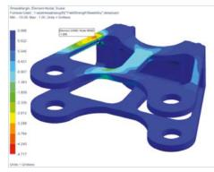
Stress margin calculation based on temperature dependent yield stress.
