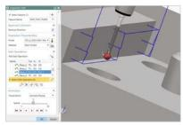
NX CMM automatically adjusts inspection paths to prevent interference with adjacent part features.
