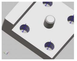
Scanning inspection paths can be automatically created by using the embedded PMI data.
