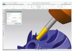
Machining high-quality impellers using a swarf operation enables precise alignment of the tool with blade geometry.
