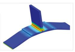
Simulation of laminate composite material showing delamination.
