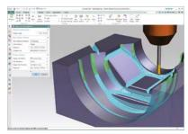
Cut region control enables precise control of rest milling tool paths.
