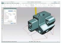
Shown is the automated chamfer milling of holes with different orientations and sizes.
