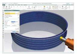
Simplified programming of complex rotary parts lets you quickly generate 5-axis tool paths.
