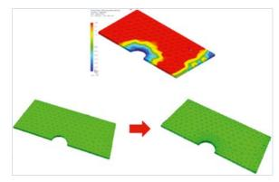
Adaptive meshing leads to better convergence and accuracy of structural, thermal and multiphysics solutions.
