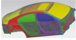
Generate fluid body models when you have mesh data but no geometry for your part or assembly.
